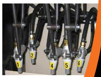
**Six or Four Blast Guns** mounted on separately adjustable holders enable operators to control blast coverage.
