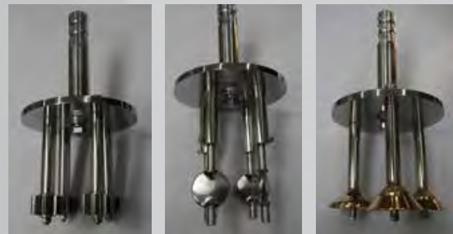
Fixtures are specifically designed to hold the process components and are attached to workstations integrated into the rotating spinner. They are partially immersed in the grinding/polishing media.
