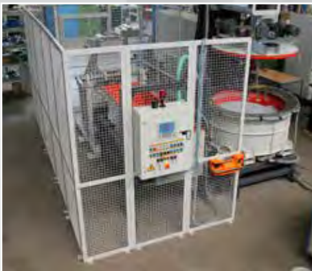
R 4/1300 SF with automatic media replenishment system
