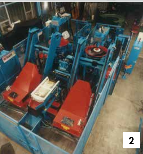
R 1/1 R plunge finisher with reciprocal rotary spindle movement
