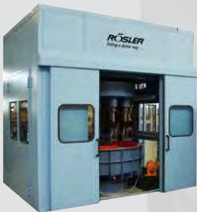
12-station system enclosed by sound attenuating enclosure
