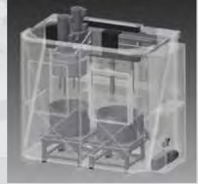
SF - mini-drag finisher for 2-stage processing
