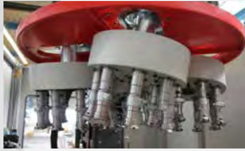
Component processing with workstation equipped with eight (8) spindles offers simultaneous processing of 32 work pieces in one batch.
