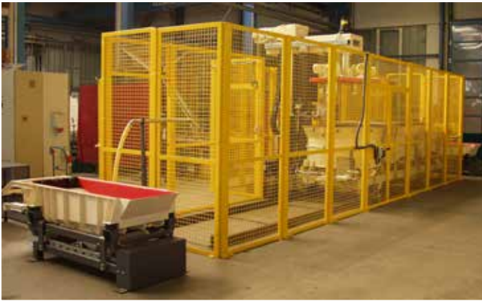
Three-station system with automatic media replenishment: Allows cut down, fine grinding and high gloss polishing without having to remove the components from the workstations.
