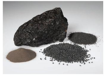
Blasting grain produced by crushing chunks of fused alumina.
