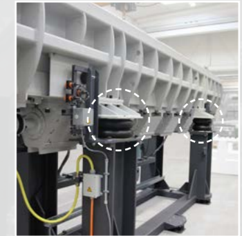
Processing bowl raised at the bowl exit - longer processing times
