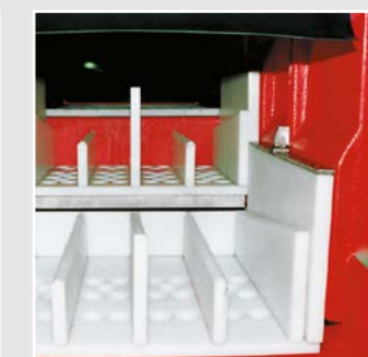
Special screen deck with tumbling steps for complex work piece shapes
