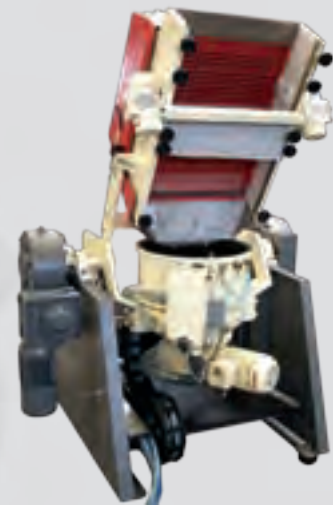
... ready for the next batch – by tilting of the separation unit the processing media is automatically returned to the work bowl.
