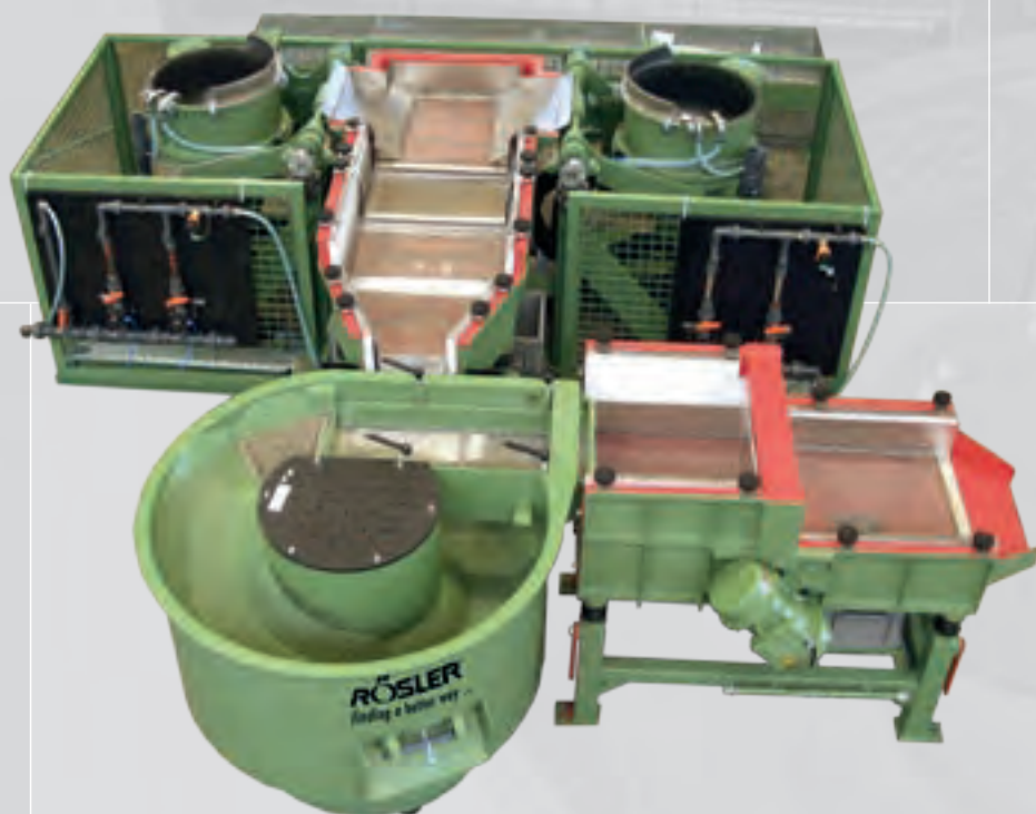
"E" tandem system – two finishing units linked to one common separation station and a rotary drier for drying and post separation.
