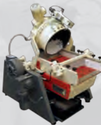
... Separation – indexing, precisely dosed discharge of the media/work piece batch from the work bowl onto the vibratory separation unit.
