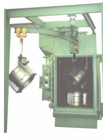
Goff Model 4860 HT shown with optional, split power doors and manual Wye Track.
