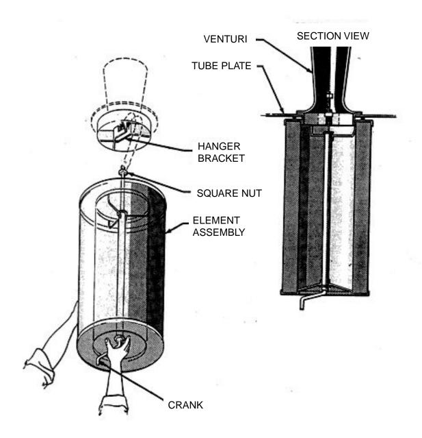
Unscrew the square nut so the top is flush with the end of the mounting rod. Insert the rod through the filter element as shown. Hang the support rod and filter on the hanger bracket. Turn the crank clockwise while holding the filter straight until the gasket on top makes contact with the tube plate. (See figure above) Tighten the filter until the gasket is compressed 50%.
