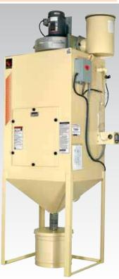
Standard Features: • Quick-release basket door • External blowoff gun • Door/blast interlock • Easily unloaded hopper door
