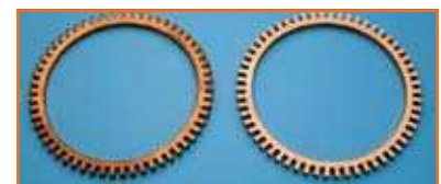
Collar deburred with glass beads
