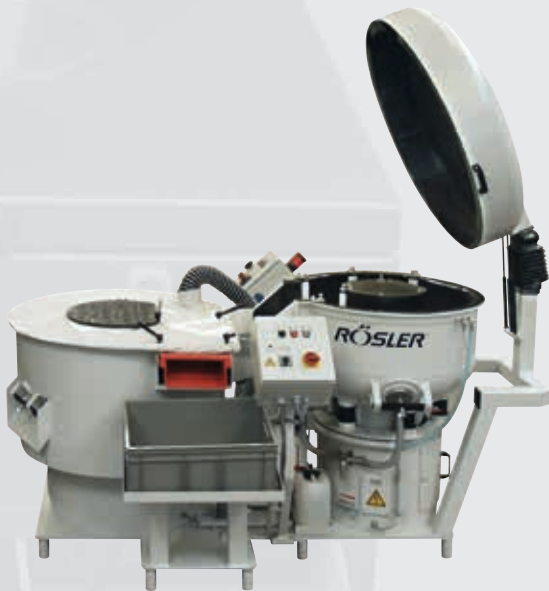
Our power package RCC1 with RCD1 – cleaning, drying and polishing of cutlery. Ideal for caterer with huge amounts.
