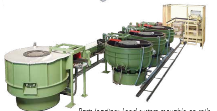
Parts loading: Load system movable on rails with integrated vibratory feed hopper conveyor belt for collecting finished parts and transferring them to a vibratory dryer
