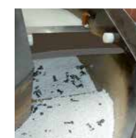
Drop behind separation flap: Prevents flat parts from sticking to each other
