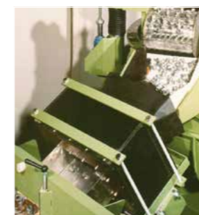
Drum magnet with de-magnetization tunnel
