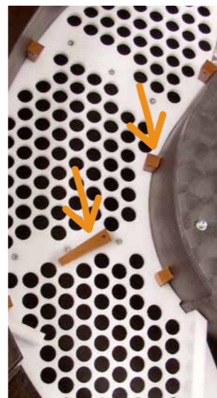
Polyurethane wedges allow quick screen fastening and exchange of screens.
