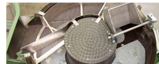
Separation screens with built-in tumbling steps Removes media from cup shaped parts
