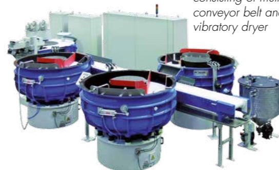
Parts loading: Load system movable on rails with integrated vibratory feed hopper conveyor belt for collecting finished parts and transferring them to a vibratory dryer
