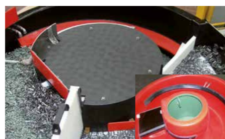
Triangular wedge profile prevents light-weight parts from sticking to the channel wall and guides them back into the media mass
