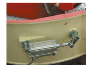
Pneumatically activated separation flap
