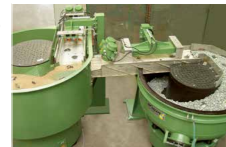
Linear separation unit with vibratory motors
