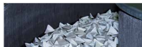
Process bowl with profiled structure: Prevents flat parts from sticking to the wall of the processing channel
