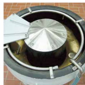
Circular rinse station in the work bowl
