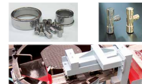
Linear separation unit with magnetic oscillator
