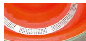
Channel screen – removal of wooden chips
