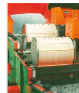
Double drum magnetic separation system for difficult to separate parts
