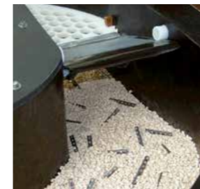
Pneumatically activated separation flap
