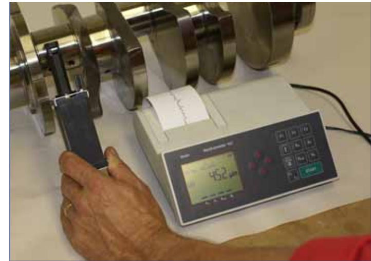
Measurable Results Specialists take RMS readings on a profilometer to measure finishing results.
